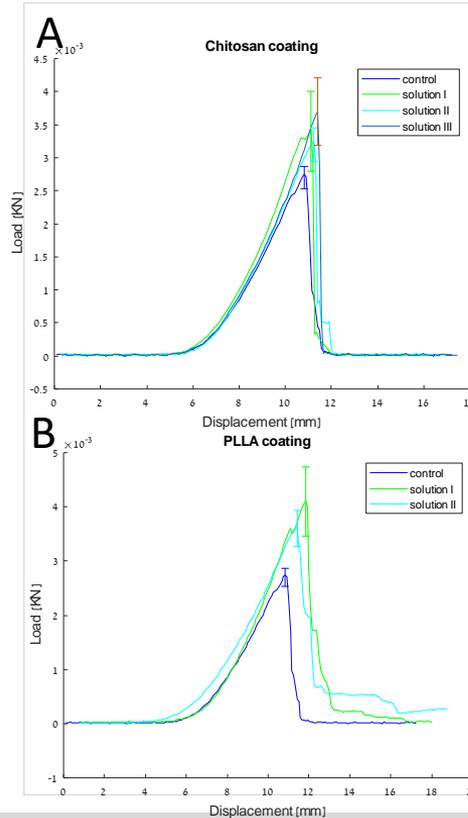
A. Load-displacement graph for mean chitosan coating (I, II & III) tensile test results compared to control group
